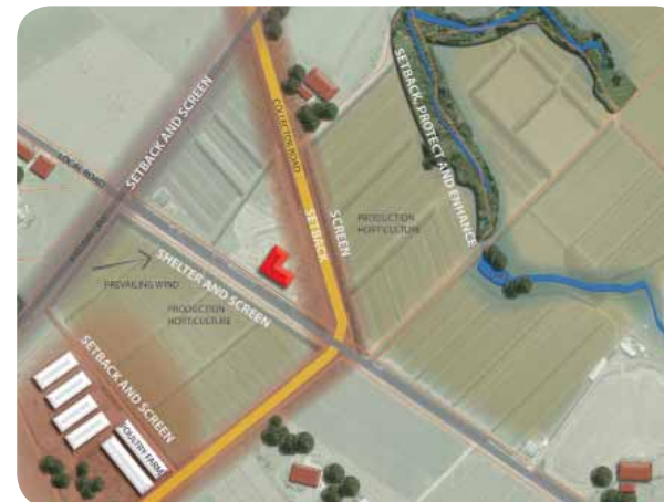
Left: Conduct a finer grain site analysis that covers greater detail for the site. Consider setting new buildings back/screening or elevating from sources of potential nuisance or reverse sensitivity that reduce living amenity including: Roads, poultry sheds, railway lines, production horticulture and streams.
