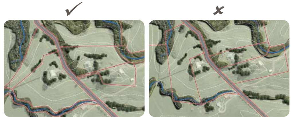
Above: Dissecting natural features with insensitive boundaries can compromise the health and amenity of the area. Alternatives include: Shared open spaces in body corporate arrangements, vesting natural features with trusts or other organisations, placing a design covenant on a feature or keeping the extent of the feature within one allotment.
