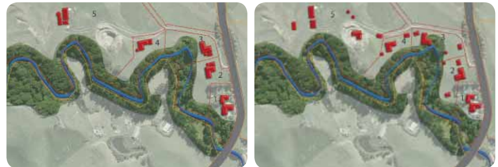
Above: Clustered buildings in combination with smaller sections and a larger balance section minimise the effect of development on the open character of the rural landscape.
