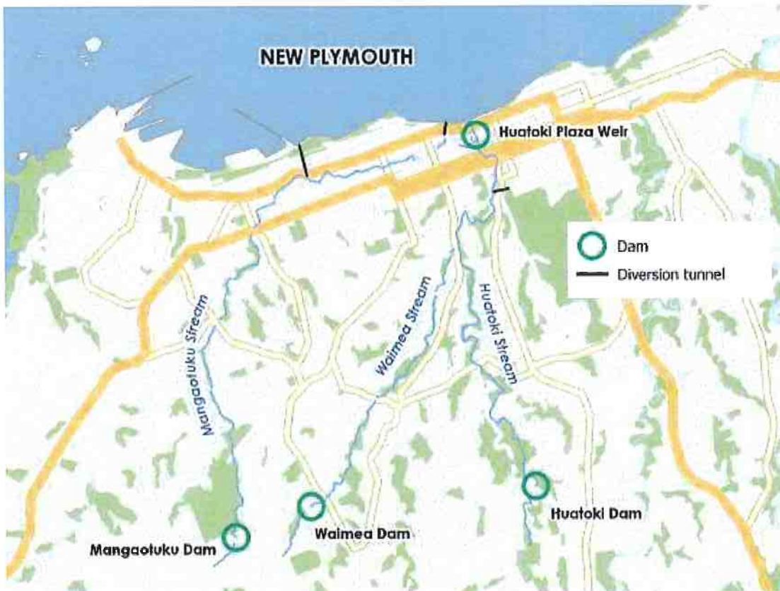
Figure 3: NPDC flood protection infrastructure
